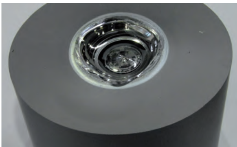
Cold monocrystalline Si brick with solidified melt following evaporation
